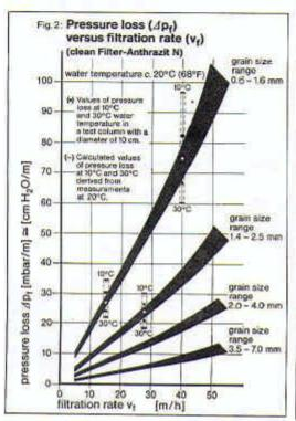
loss increases with increasing loading i.e. it is proportional to the total amount of matter retained in the litter. Backwashing removes the substances retained by the filter and the pressure loss in the clean filter is restored. to the original value. The pressure loss dp, in a 1 m layer of clean Filter-Anthrazit N in relation to the filtration. rate is shown for the different grain size ranges in figure 2.
