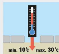
During joint filling and during the first days of hardening, the air and soil temperature must be at least 10 ° C.
