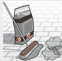
Sweep the filling material into the joints using a soft broom. Sweep lengthwise and diagonally on the joints until they are completely filled.
