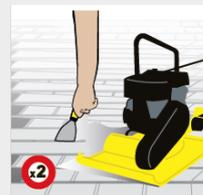
Compact the joints using a vibrating plate - do this at least twice. Use a protective rubber mat to protect the paving. Check that the joint is fully compacted - use a spatula. You should only be able to press the spatula one or two mm into the joint.
