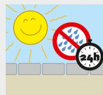
Both the weather and the substrate must be dry for the joint to harden completely. The joint does not withstand rain (except fine drizzle and dew) for the first 24 hours.
