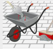
Check the weather forecast before beginning to work. Mix the contents in a mason jar or a wheelbarrow so that the binders are mixed with the silica sand. Never mix the contents of more than two bags at a time.
