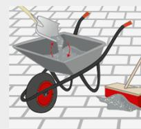
Mix the contents of a mason jar or a wheelbarrow so that the mineral additives and binding agents are mixed well with the silica sand. Mix the contents from a maximum of two sacks at a time.
