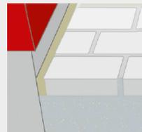
**NOTE!** Avoid using the material in the joint directly adjoining the plinth as there is a risk of expansion damage and efflorescence. Use laying sand or something else in the joint adjoining the plinth.
