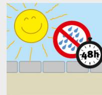
Before you start filling the joints, please ensure that the pavement and joint filling material are completely dry. Otherwise, the binding agents may stick to the surface of the paving and form a greyish residue. Additionally, please check the weather forecast, as the joints should not be exposed to rain for the first two days.
