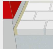
Check that the joint is compacted well using a spatula. You should not be able to press the spatula more than a few millimetres into the joint. Refill if necessary and sweep the paving surface clear of filling sand.
