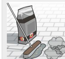
Sweep the filling materials into the joints using a soft broom. Sweep in a diagonal pattern until the joints are filled to the top.
