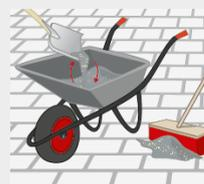
Mix the filling material in a bucket or a wheelbarrow using a shovel to mix the mineral additives with the silica sand. Never mix the contents from more than two bags at a time.
